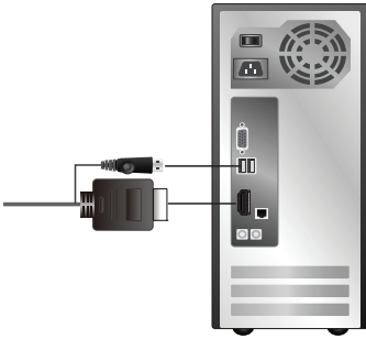
USB KVM Cable Connection
